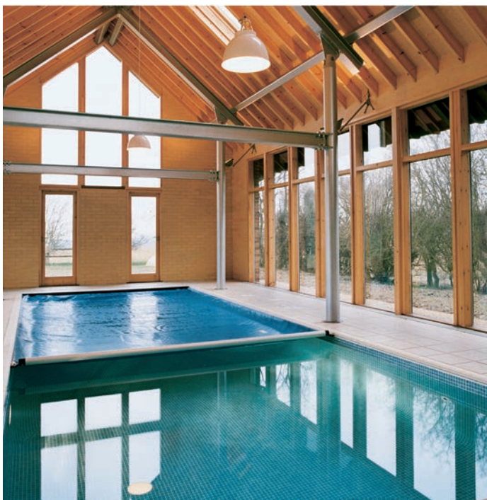
For indoor pools, a cover provides the added benefit of eliminating the need for expensive dehumidification systems.
