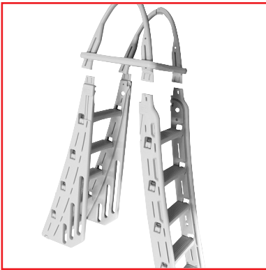
#4: Align the inside/outside rails with deck/handrail.
